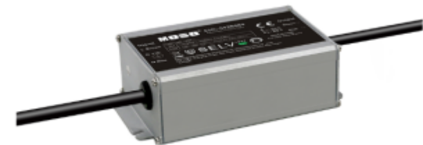
MOSO PSU: 0.7A/30-60V, CC, metal case, rectangular
